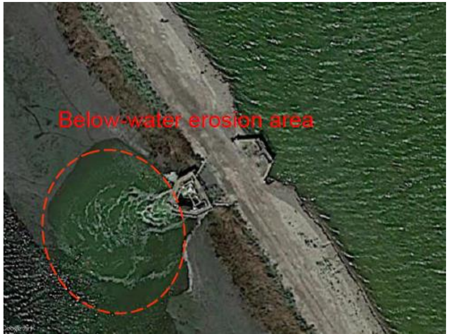
Google Earth satellite imagery details the erosion on the outboard side of the southern hydraulic structure.
