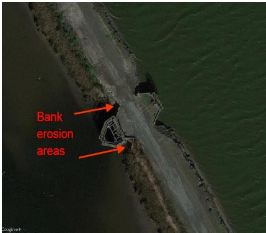
Google Earth satellite imagery details the erosion on the outboard side of the southern hydraulic structure.
