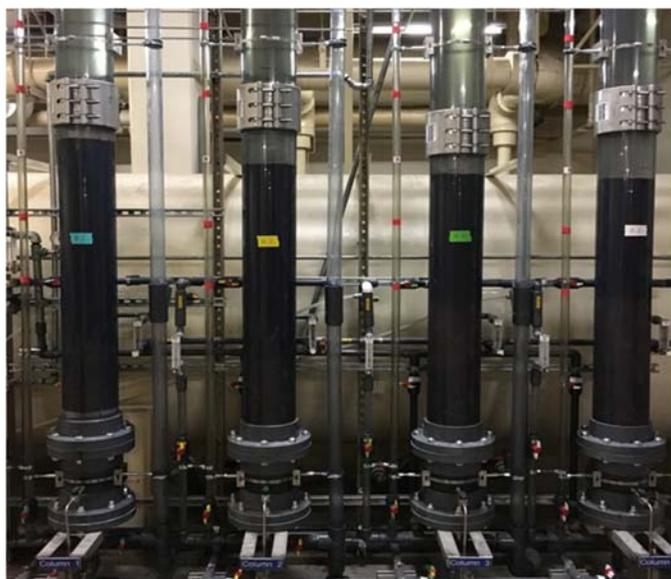
Figure 3: Four various filter media configurations tested.
