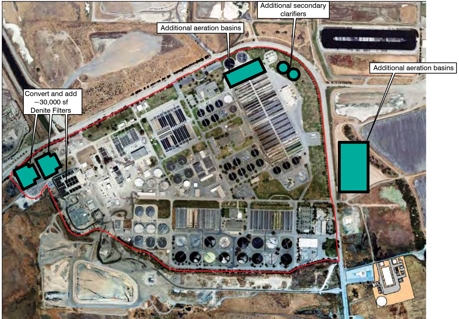
Figure E-10 FOOTPRINT REQUIREMENT FOR ALTERNATIVE 2 (TN < 3 MG/L) SAN JOSÉ/SANTA CLARA WPCP MASTER PLAN CITY OF SAN JOSÉ
