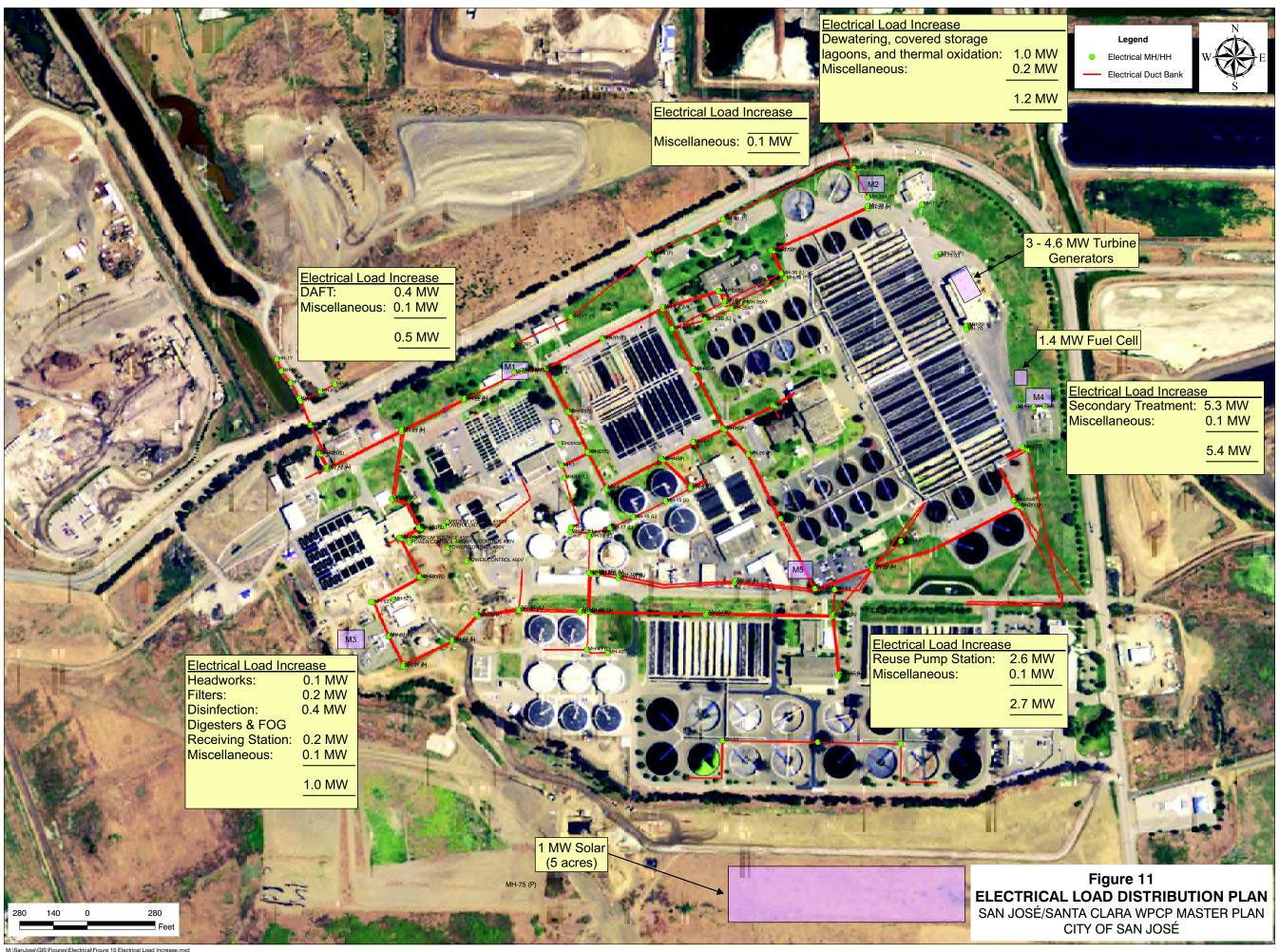
The plant is currently in the process of a major electrical distribution system upgrade, including the improvements necessary to convert the existing 4.16 kilovolt (kV) electrical distribution system into a ring bus system<sup>3</sup>. The power increases are grouped and shown on the figure relative to the nearest switchgears (M1 through M5).
