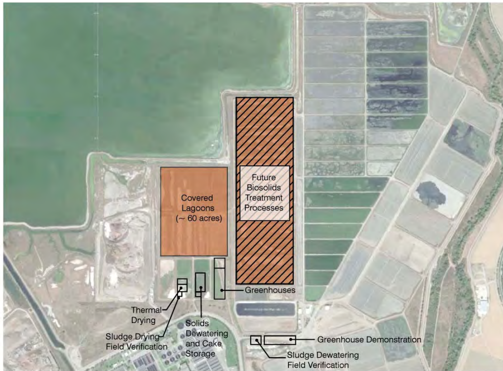
Figure 7 FOOTPRINT REQUIREMENTS FOR 2040 SAN JOSÉ/SANTA CLARA WPCP MASTER PLAN CITY OF SAN JOSÉ
