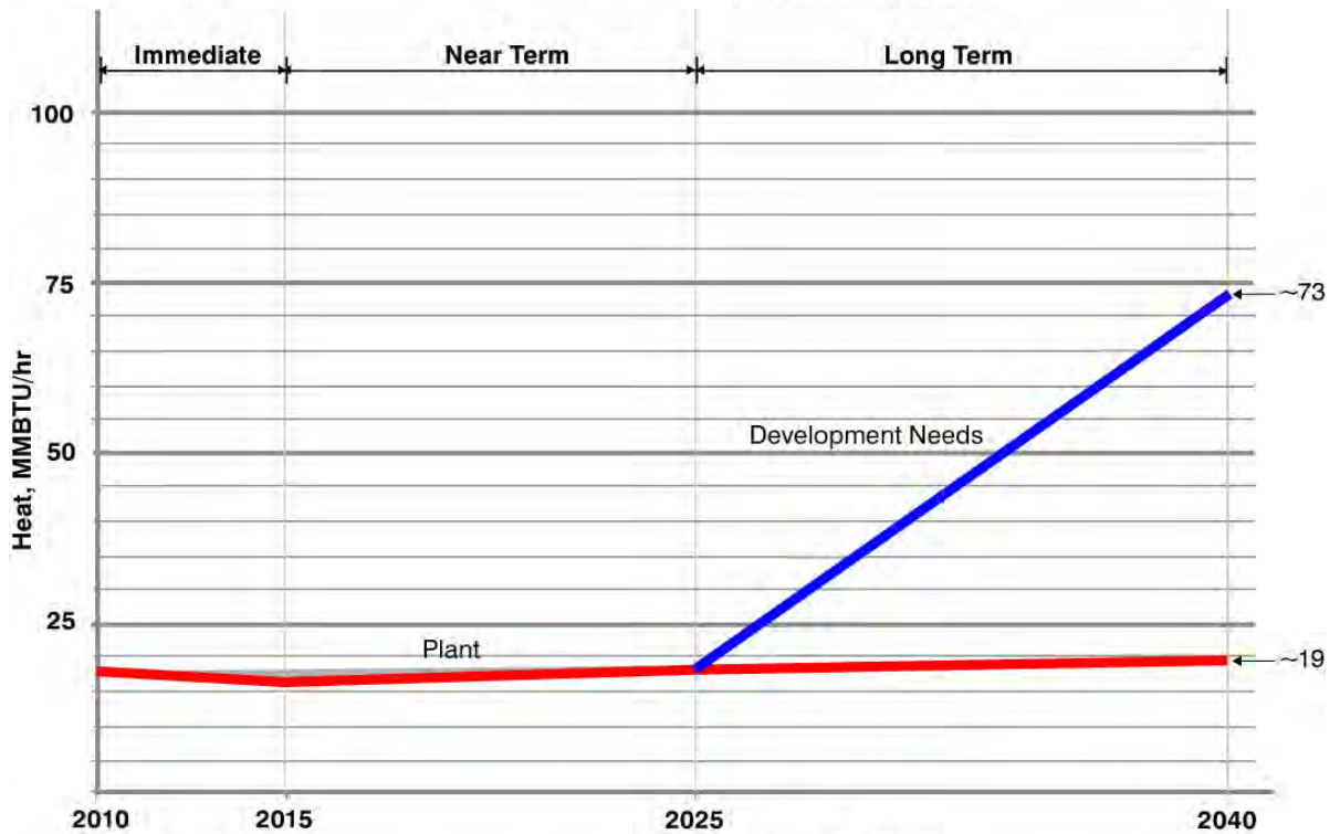
Figure 16 WPCP AND COMMERCIAL DEVELOPMENT HEAT DEMAND SAN JOSÉ/SANTA CLARA WPCP MASTER PLAN CITY OF SAN JOSÉ
