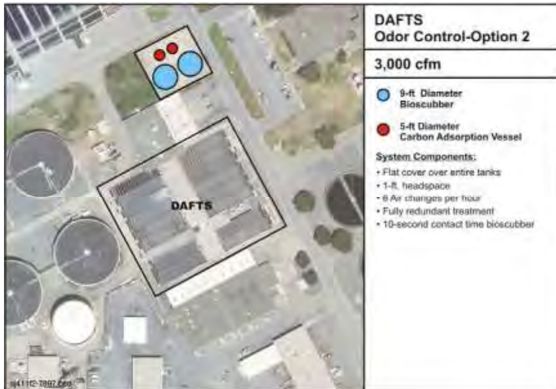
Figure G-8 DAFTs Bioscrubbers + Activated Carbon
