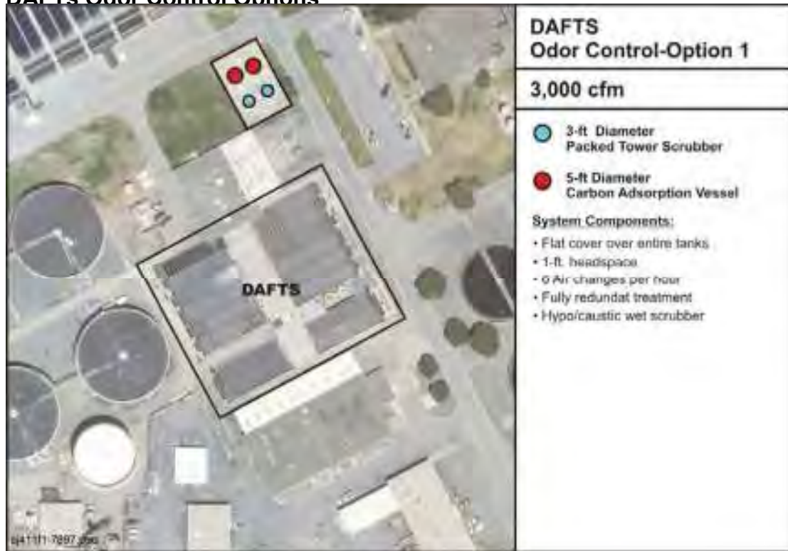
Figure G-7 DAFTs Packed Tower Scrubbers + Activated Carbon
