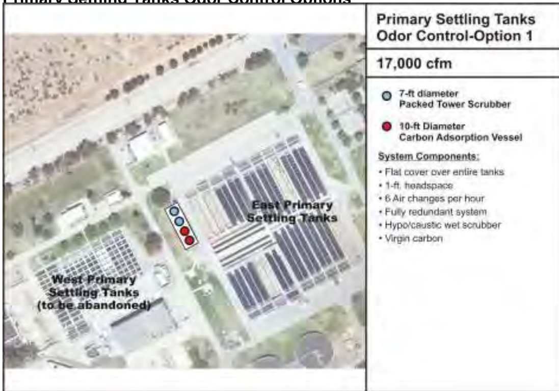
Figure G-4 Primary Settling Tanks Packed Tower Scrubbers + Activated Carbon
