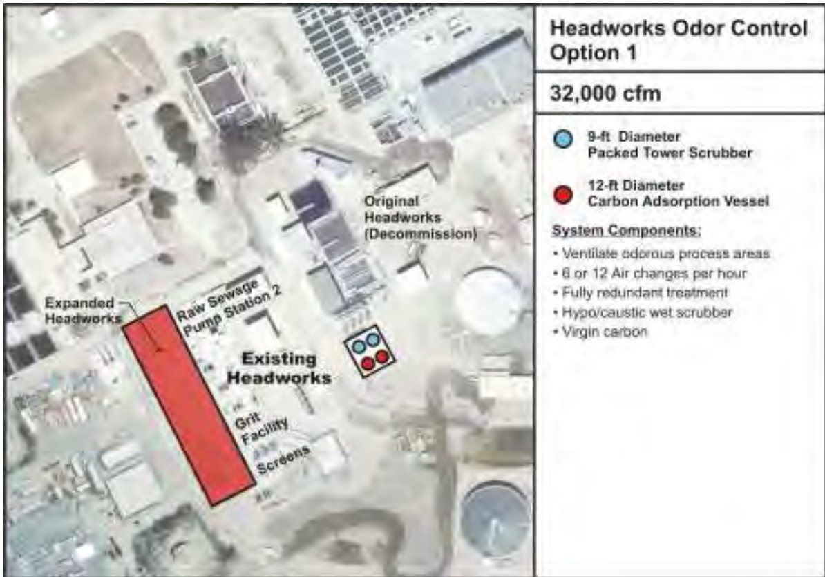
Figure G-1 Headworks Packed Tower Scrubbers + Activated Carbon
