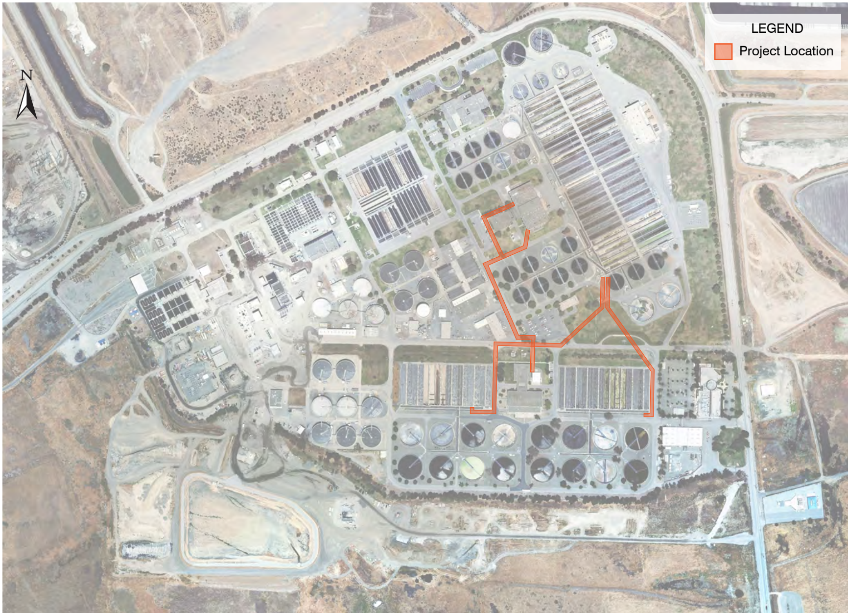
Figure 18 CONNECT BNR 1 AND BNR 2 CLARIFIERS SAN JOSÉ/SANTA CLARA WPCP MASTER PLAN CITY OF SAN JOSÉ
