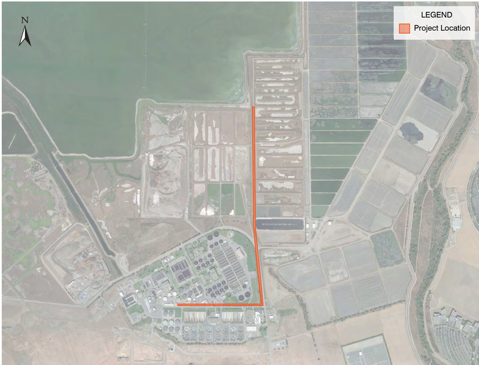
Figure 57 14-INCH DIGESTED SLUDGE LINE ADDITION SAN JOSÉ/SANTA CLARA WPCP MASTER PLAN CITY OF SAN JOSÉ
