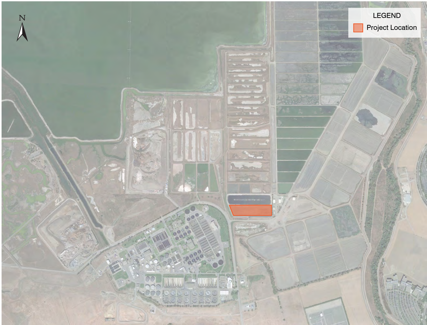
Figure 16 ADDITIONAL 12 MG PE EQUALIZATION BASIN SAN JOSÉ/SANTA CLARA WPCP MASTER PLAN CITY OF SAN JOSÉ
