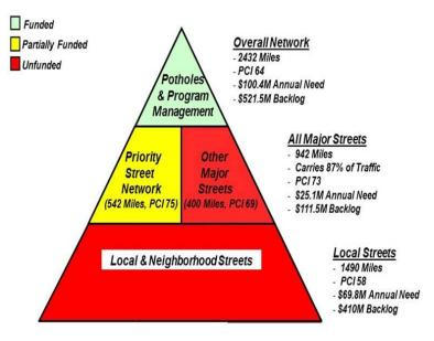
PCI = Pavement Condition Index Ratings: Good (100 to 70); Fair (69 to 50); Poor (under 50)
