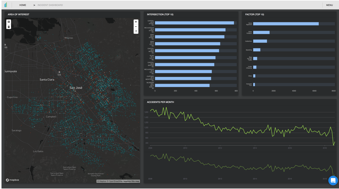
Figure 13: Home interface of the incidents dashboard developed using the incidents data delivered to UrbanLogiq. Here, the user can see each intersection coloured by the number of incidents that occurred there during the chosen time period. Intersections with more incidents are coloured red, while those with fewer incidents are coloured white. The top middle and top right panels rank intersections and incident factors by the number of associated incidents, respectively. The time series plot towards the middle shows how the number of incidents has changed over time, while the curve beneath it allows the user to select a particular time period for analysis and display.
