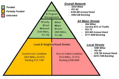
PCI = Pavement Condition Index Ratings: Good (100 to 70); Fair (69 to 50); Poor (under 50)
