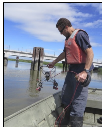
FIGURE 54 BRYAN FRUEH DEPLOYING A CONTINUOUS WATER QUALITY METER IN COYOTE CREEK
