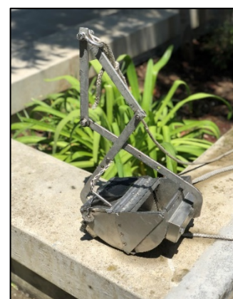
FIGURE 58 PETITE PONAR SEDIMENT GRAB FOR BENTHIC SAMPLING
