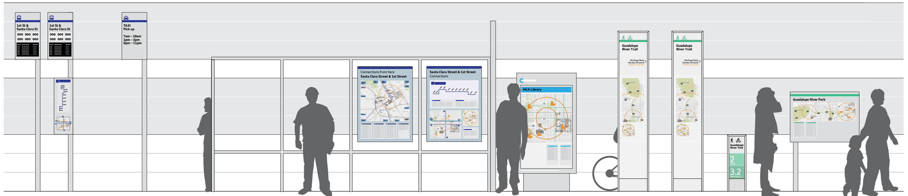
Standard stop flag Face A Taxi flag Face A/B Transit shelters (Types TBD) Transit shelters (Types TBD) Bike share product Trail map product Face A Face B Route marker Park product
