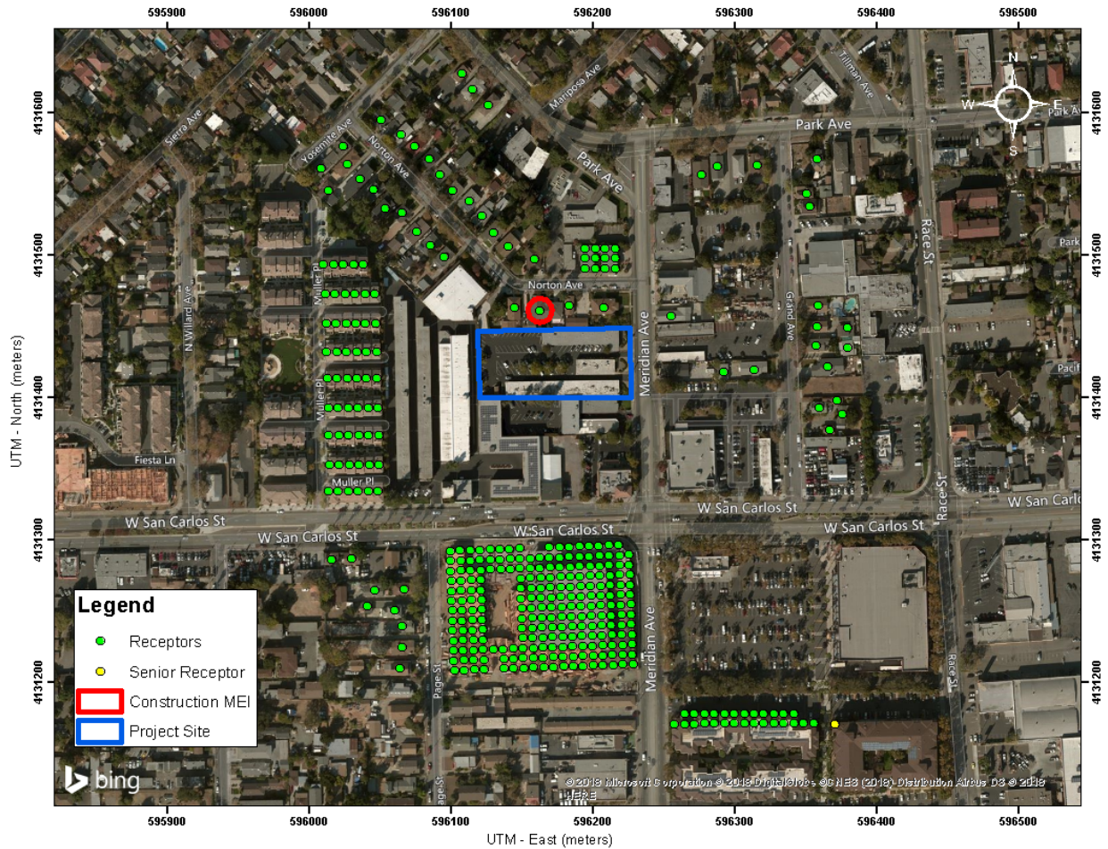
Figure 2. Project Construction Site and Locations of Off-Site Sensitive Receptors and Maximum TAC Impacts
