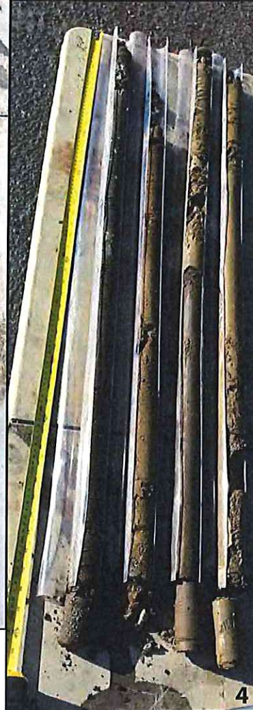
Photo 1. Overview of west side of Project APE at Core 6 with Tim Tyler at truck rig and Donielle Neddeau taking notes, view to north with one of the gates beyond. Photo 2. Overview of Project APE drilling Core 2, view to south. Photo 3. Soil samples from Core 5 with top in upper right. Photo 4. Soil samples from Core 5 with top in upper right.
