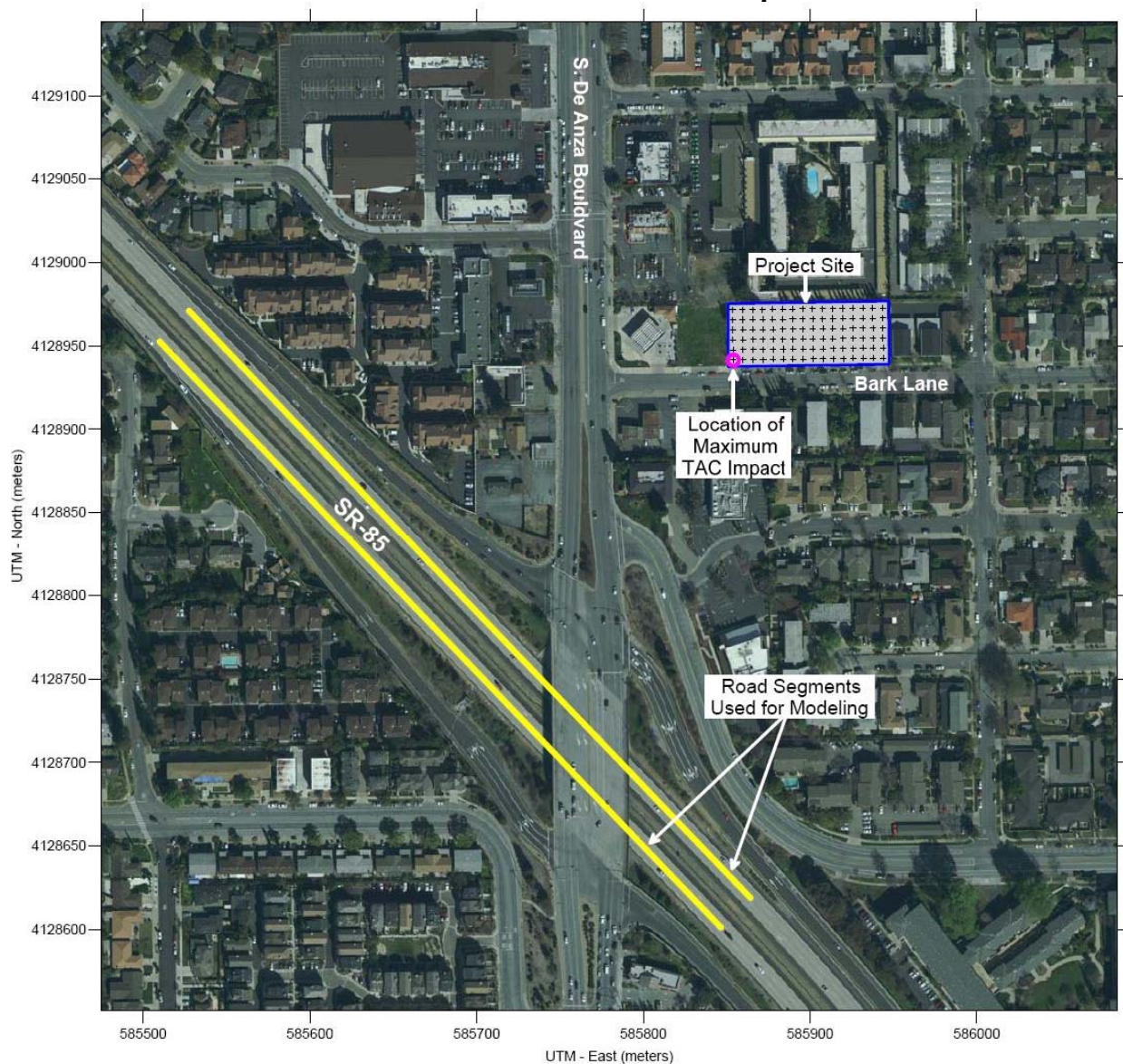
Figure 2. Project Site and On-site Residential Receptors, Road Segments Evaluated, and Locations of Maximum TAC and PM 2.5 Impacts
