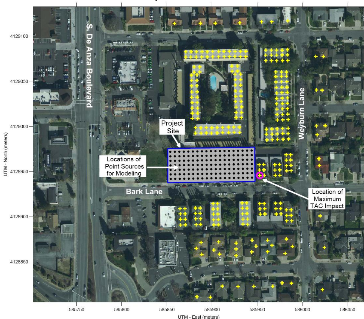
Figure 3. Project Construction Site and Locations of Off-Site Sensitive Receptors and Maximum TAC Impacts
