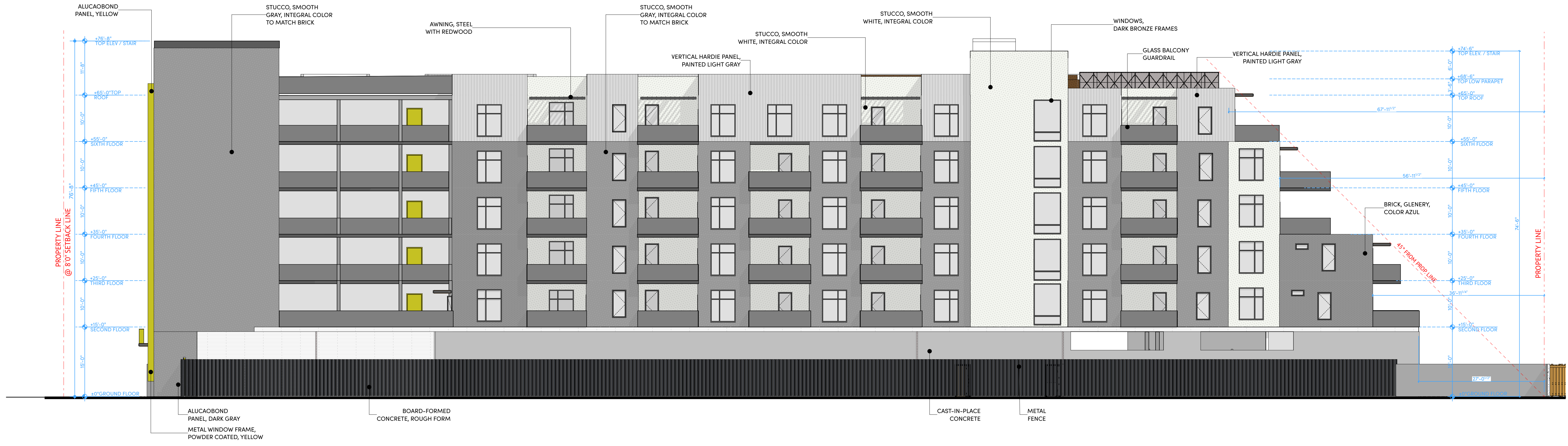
2 NORTH ELEVATION SCALE: 3/32" = 1'-0"
