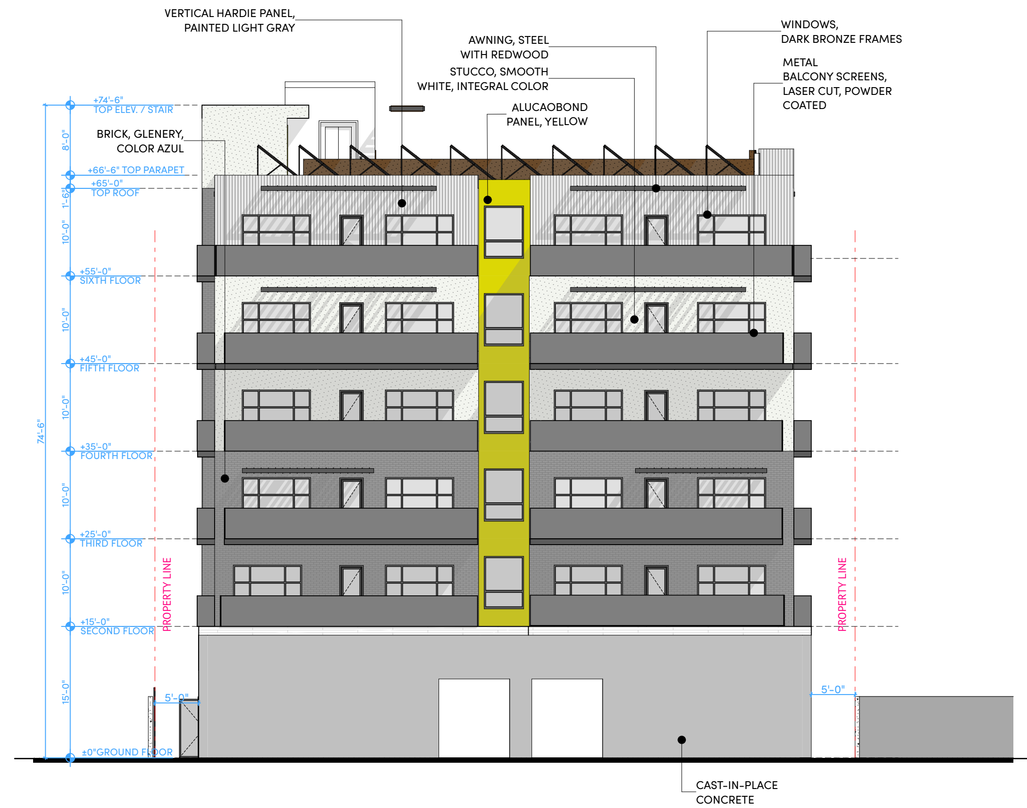
1 WEST ELEVATION SCALE: 3/32" = 1'-0"
