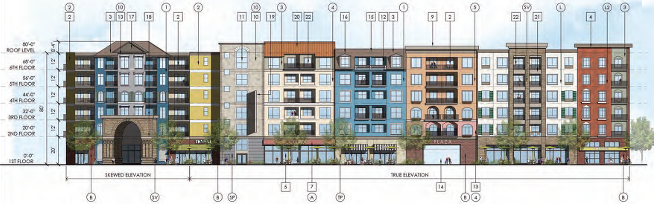
1 WEST ELEVATION (UNION AVENUE) 1" = 20'-0"
