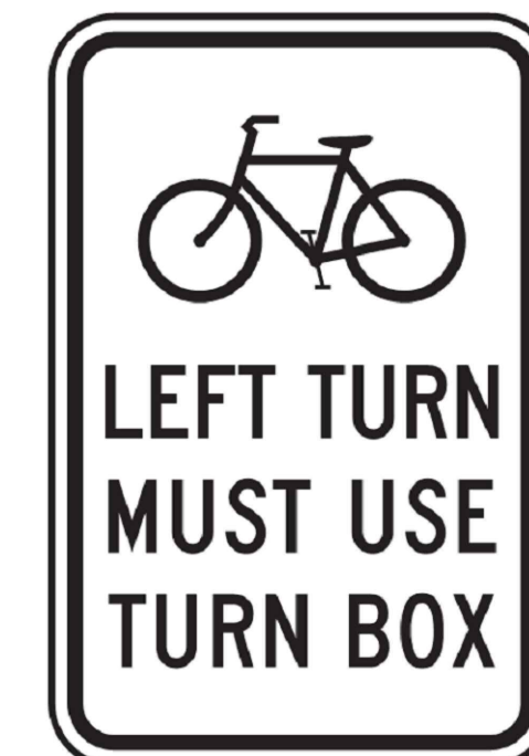
R (SPECIAL) "LEFT (RIGHT) TURN MUST USE TURN BOX" R9-23aL (12" X 18") DETAIL J1 NTS
