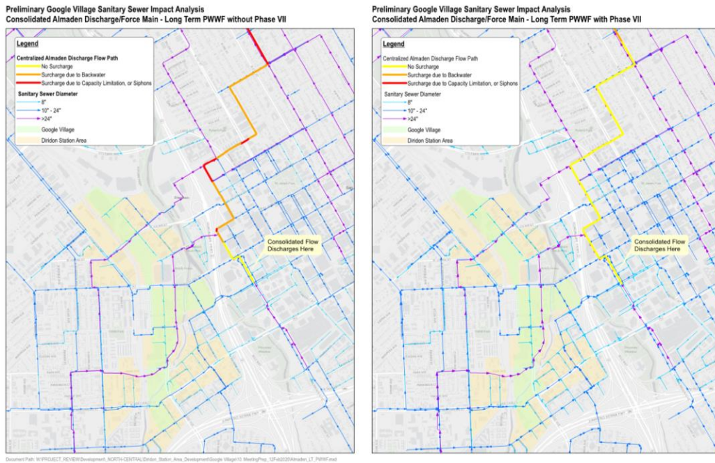
Figure 7.3. Scenario 1, One or Two WRFs with one point of connection along Almaden Boulevard
