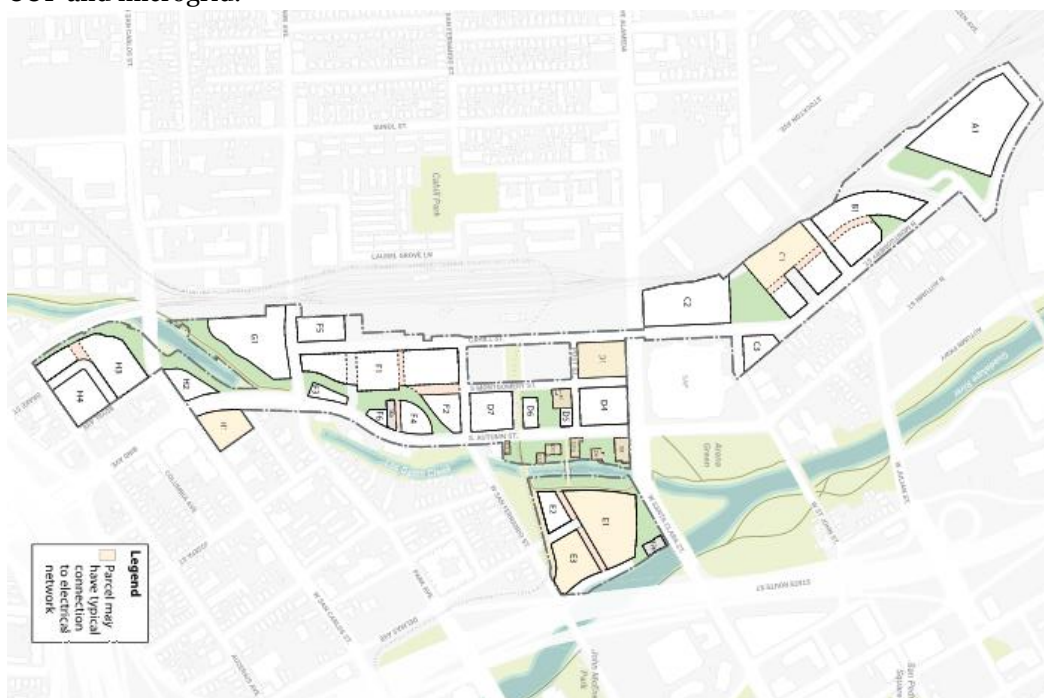
Figure 9.7. Locations of buildings which may be provided with power from PG&E directly instead of the CUP and microgrid.
