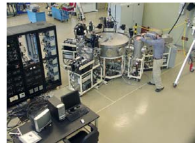
National Renewable Energy Laboratory, Silicon cluster tool at the Process Development and Integration Laboratory
