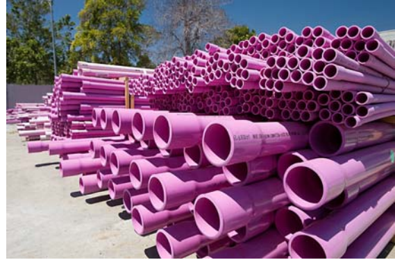
Recycled Water Purple Pipes
