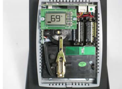
Wireless Pneumatic Thermostat. Photo courtesy of Cypress Envirosystems.
