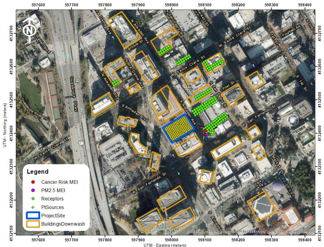
Figure 1. Project Construction Site, Building Downwash, and Locations of Point Sources, Off-Site Sensitive Receptors, and Maximum TAC Impacts
