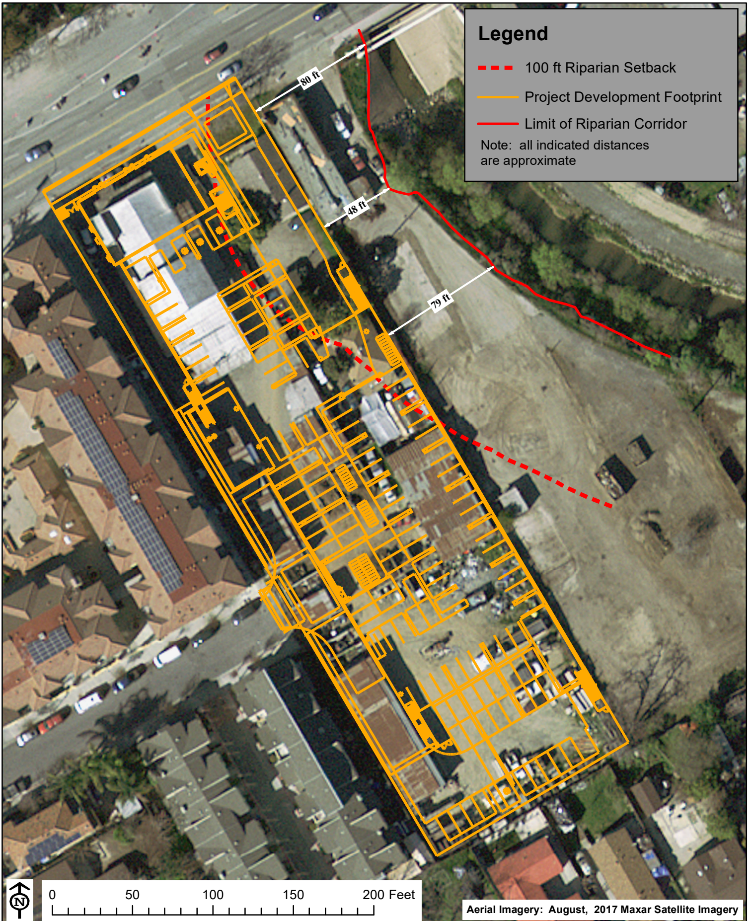
Figure 6. Riparian Corridor Setback Distances Between Project Development and the Riparian Corridor Limit of Lower Silver Creek 1936 Alum Rock Avenue, San Jose, Santa Clara County, California
