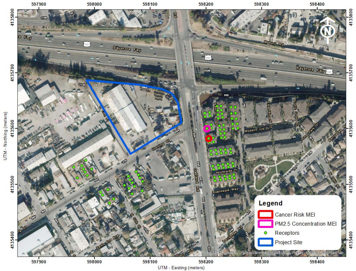
Figure 1. Project Construction Site, Locations of Off-Site Sensitive Receptors, and TAC Impacts
