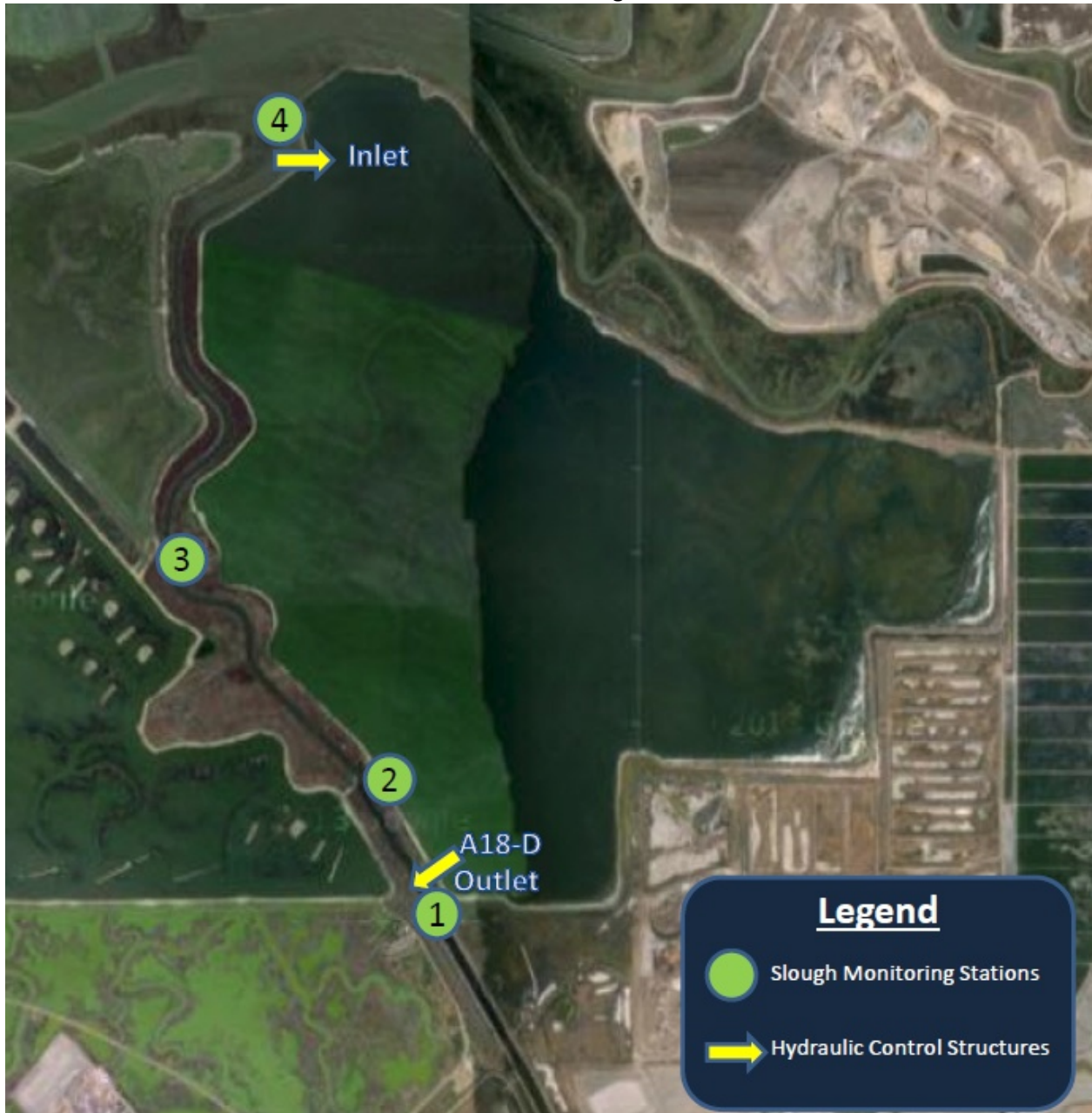
Figure 1. Artesian Slough and A18 Monitoring Stations and Hydraulic Control Structures Arrows indicate the current directional flow of water through the water control structures.
