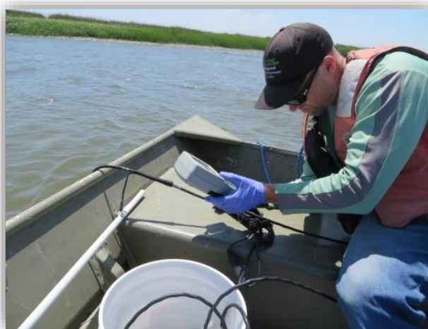
Ryan Mayfield records water quality measurements using a multi-probe YSI.
