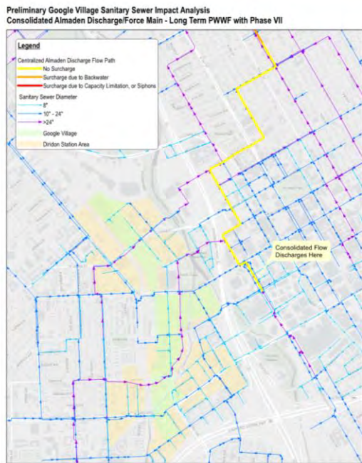
Figure 7.3. Scenario 1, One or Two WRFs with one point of connection along Almaden Boulevard
