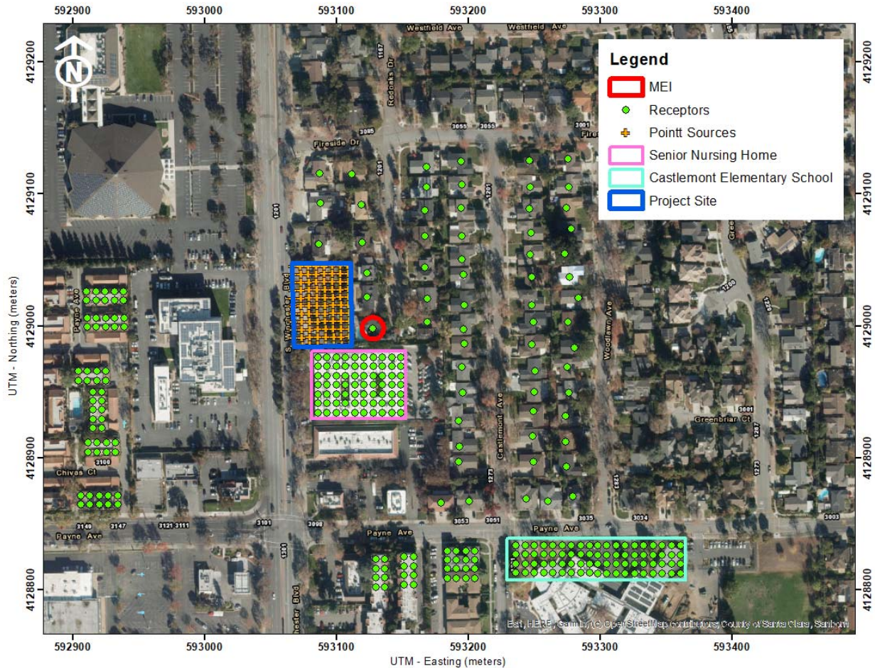
Figure 1. Project Construction Site, Locations of Modeled DPM Point Sources, Locations of Off-Site Sensitive Receptors, and Maximum TAC Location
