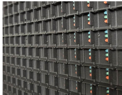
Figures 1 and 2. Close up photographs of SITELINE module face viewed from front (left) and from side (right). Note the red, green and blue diode lenses are directly visible from front direction but are obscured behind baffles viewed from the side.
