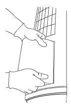
Install the new door assembly with the key lock by bowing the door with both hands and aligning the door hinge pins with their bracket in the front. (Figure 26)
