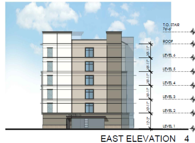
Exterior Elevations - Building B
