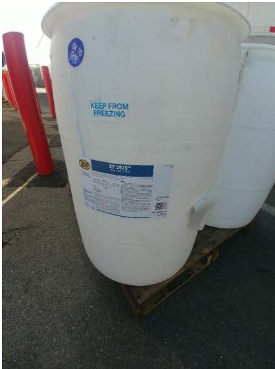
Photograph 10. The solution is stored in 55-gallon polyethylene drums which are palletized.
