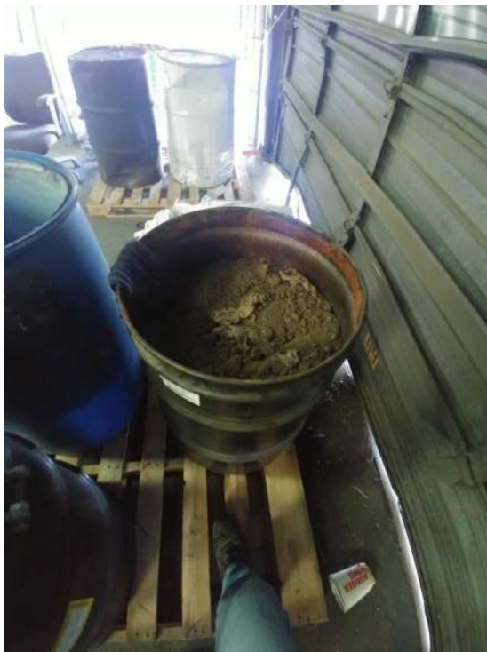
Photograph 24. Approximately five 55-gallon drums (four steel, and one polyethylene) containing motor oil, used oil, and the pictured drum which contains soil. The soil did not appear stained, and did not have an odor.
