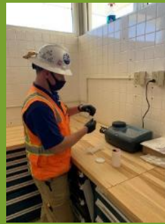
Contractor functional testing a meter.
