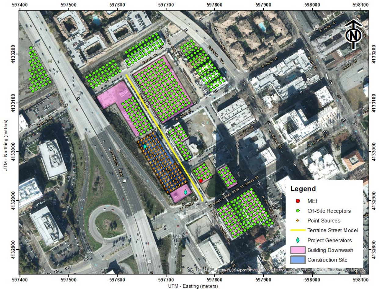
Figure 1. Locations of Project Construction Site, Modeled DPM Point Sources, Project Traffic, Project Generators, Buildings Evaluated for Downwash Effects, and Maximum TAC Location (MEI)
