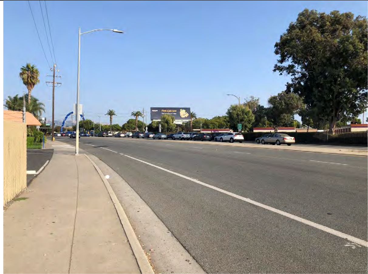
Tully Rd, facing E towards intersection with S. 7 th St. Note: broad curve of Tully Rd and fast speed of traffic causes visibility issues for driveway egress.
