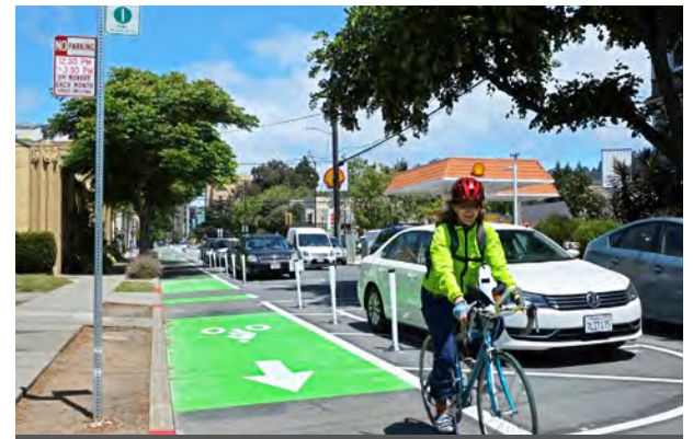
Protected Bicycle Lane Shielded by Parking
