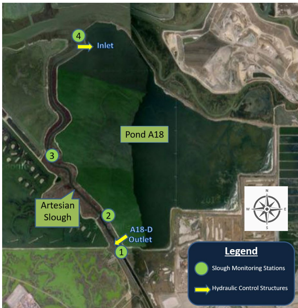
Figure 1. Pond A18 monitoring stations and hydraulic control structures- Southern Discharge. Arrows indicate the flow of water through the control structures
