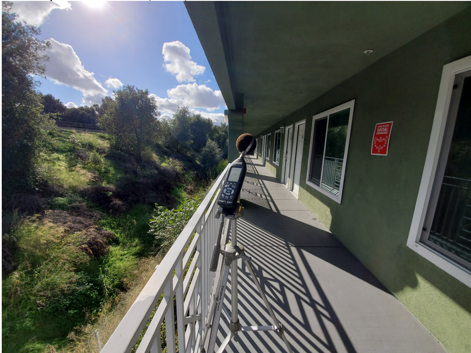
Figure 3: Microphone Position at ST-1a (Exterior)
