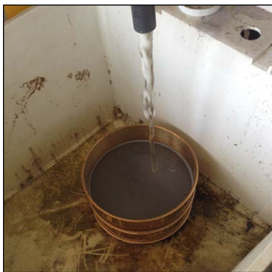
Seive collecting a 2-hr grab sample for measuring microplastics in RWF final effluent.
