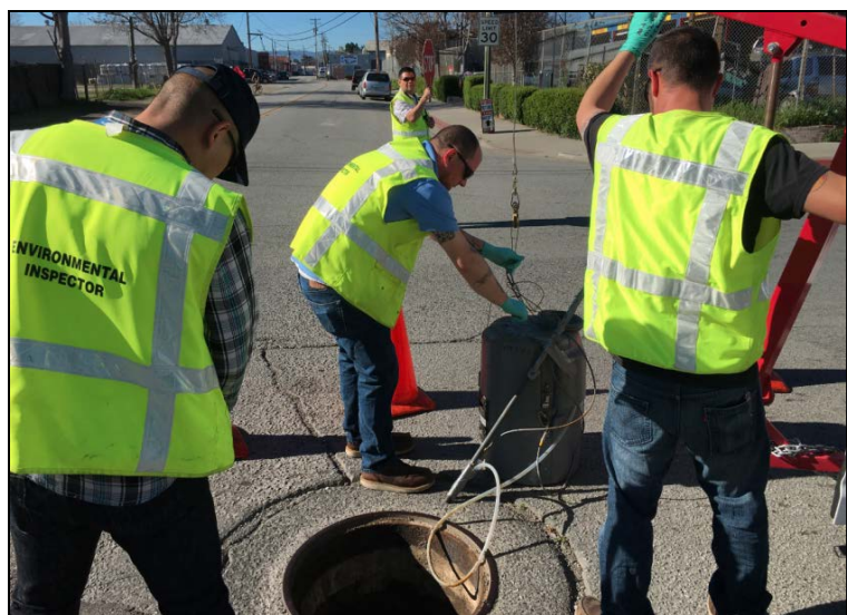
Inspectors Isaac Tam, John Fosnaugh, and Chris Fivecoat set up an automatic sampler to investigate pollutant sources.
