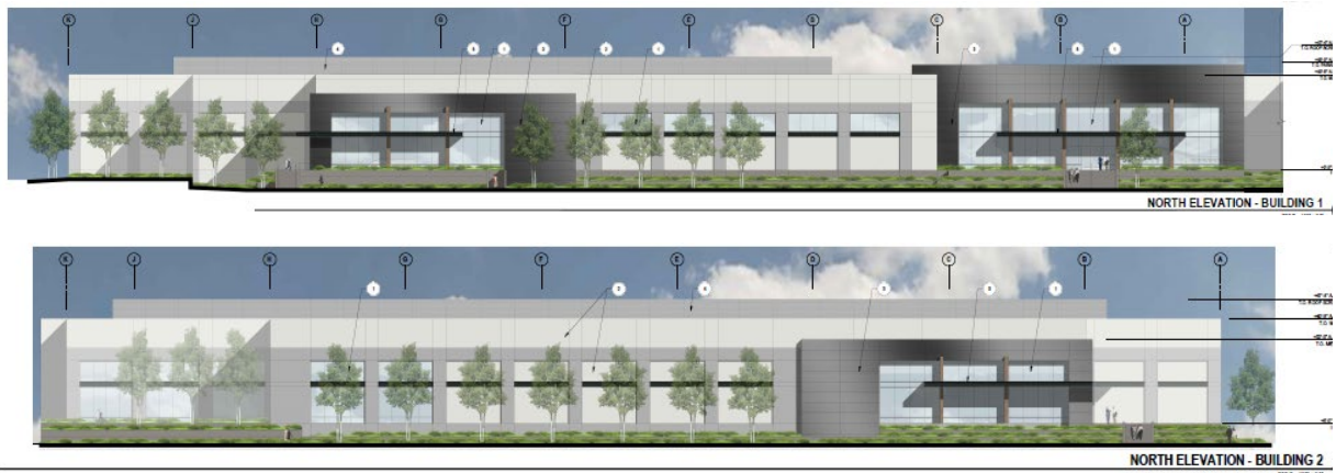
Exhibit 1. The north façades of Buildings 1 and 2 have moderate amounts of glazing, which incorporates overhangs and vertical columns, making it more visible to birds.
