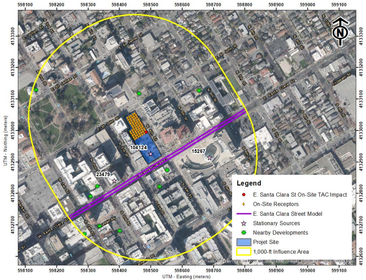
Figure 3. Project Site, On-Site Residential Receptors, Roadway Segments Evaluated, and Locations of Maximum Roadway TAC Impacts
