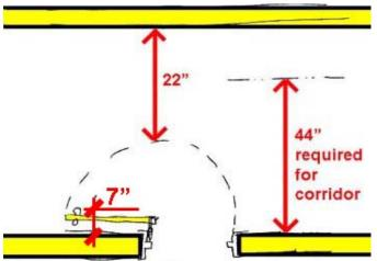
Doors swing in direction of means of egress (except where occupancy is low, i.e., less than 50
