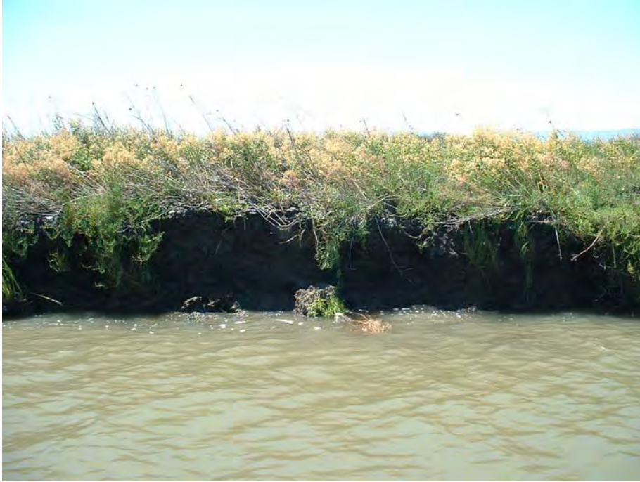
Figure F-5. Scour Along Marsh Edge Along Coyote Creek (Triangle Marsh (Segment 11)).
