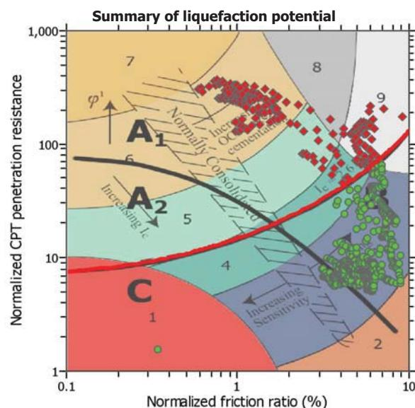
Zone A<sub>1</sub>: Cyclic liquefaction likely depending on size and duration of cyclic loading
