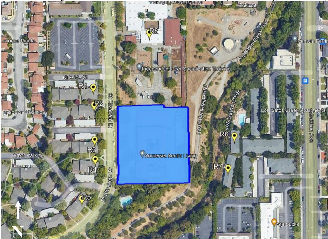
The construction noise levels were calculated to range from 73 to 86 dBA  $L_{eq}$  at 50 feet, using FHWA’s Roadway Construction Noise Model (RCNM), which assumes that all the equipment could be operated simultaneously, for a worst-case scenario. At the closest residence (R3) located about 220 feet to the west (along St. Elizabeth Drive), hourly average noise levels are calculated to range from about 60 to 73 dBA  $L_{eq}$  (as shown in Table 7).
