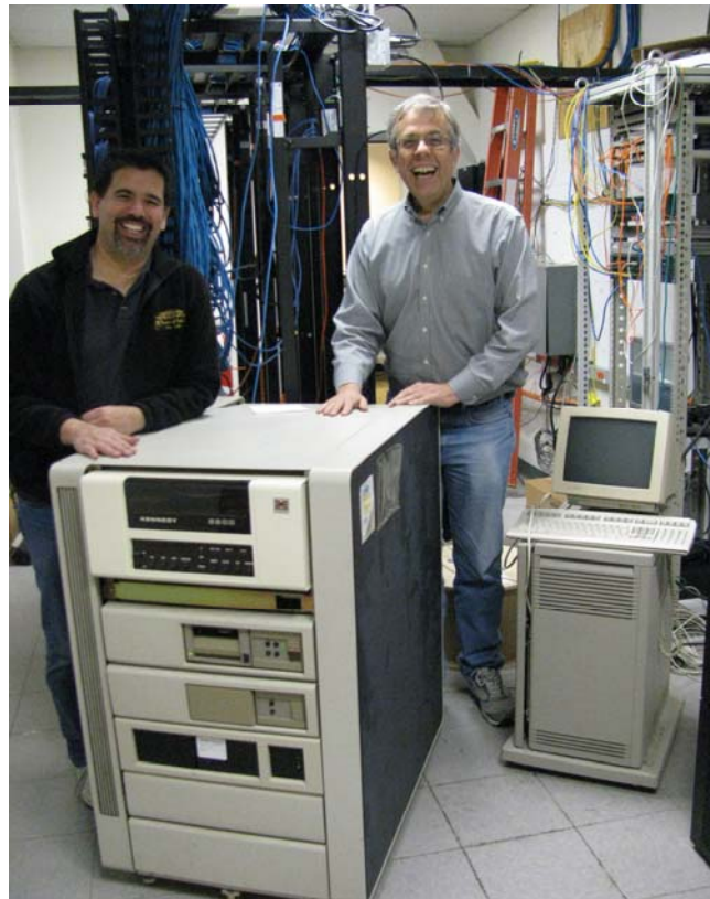
The old VAX was comprised of two units: Microvax II in the large tower (purchased in 1987) and VAX 4000-300 in the smaller tower (purchased in 1990).
