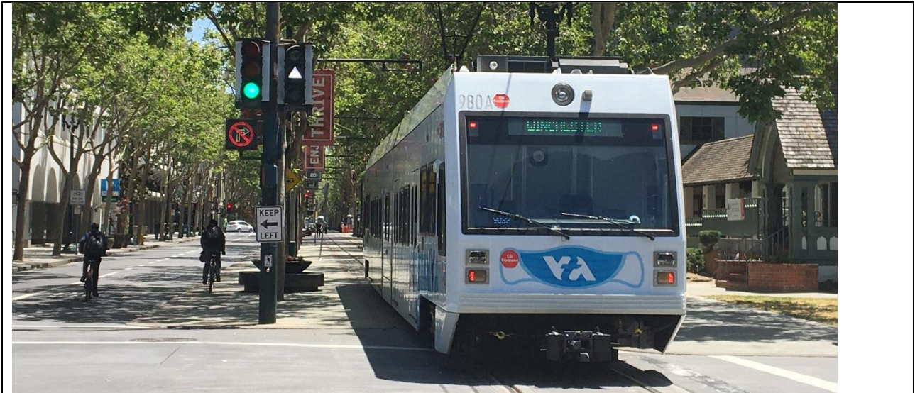
A Transit Priority Signal (White Symbol Right of Traffic Light) Gives a LRT Vehicle Permission to Enter the Intersection Before Autos, Downtown San José
