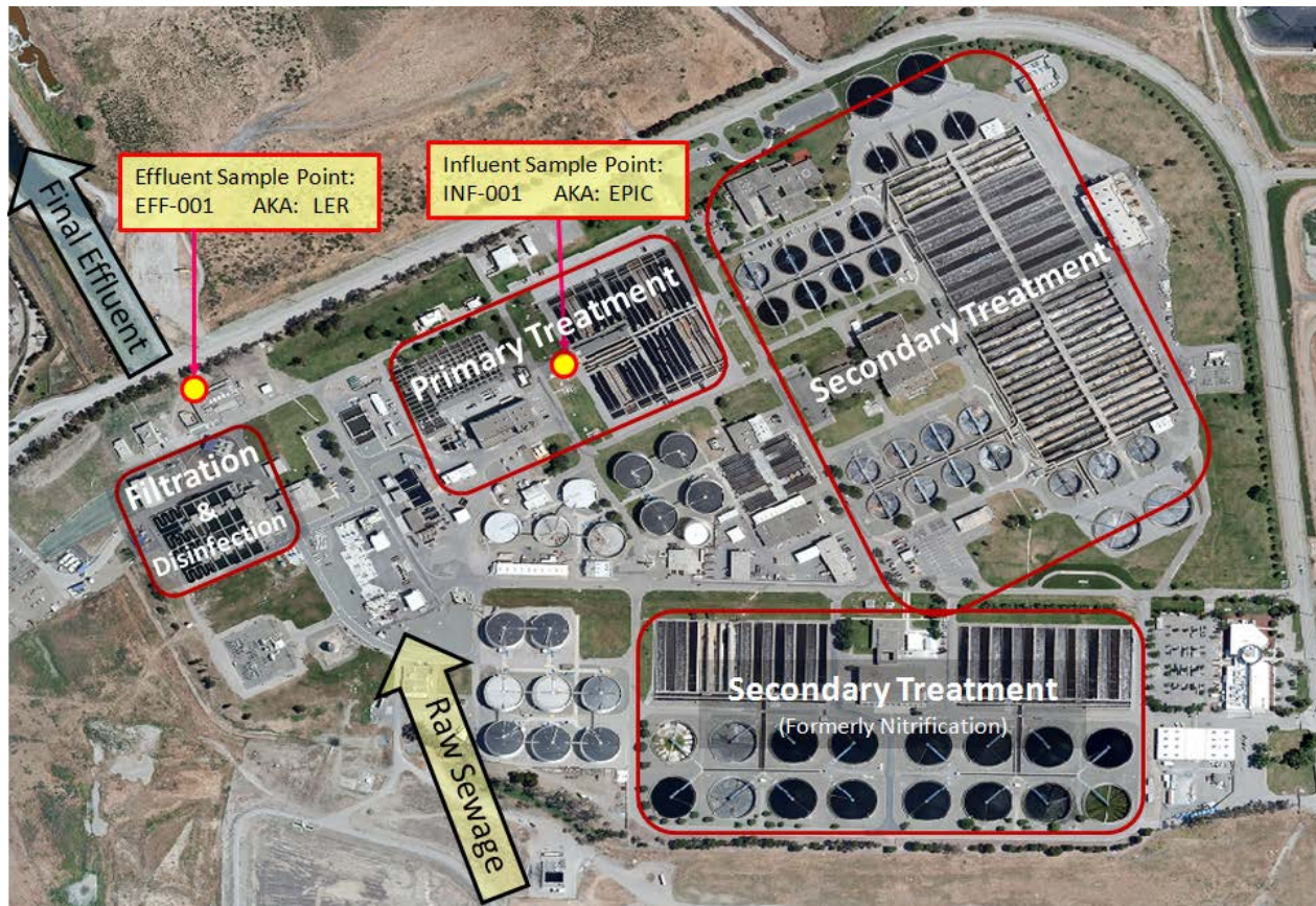
Water Pollution Control Plant: flow routing and influent and effluent sampling stations.
