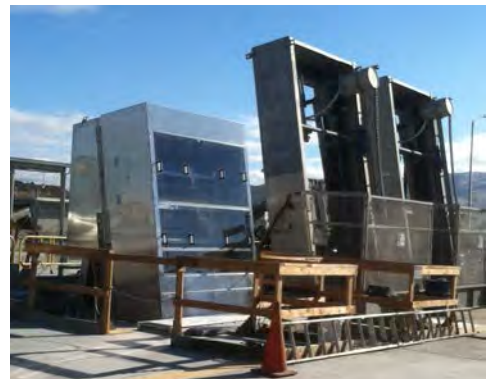
HW2 bar screens: Duperon Flex Rake at left, two traditional bar screens on right.
